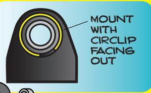
MOUNT WITH CIRCLIP FACING OUT
