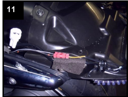
Using supplied Posi-Lock™ connectors from kit install connectors from old turn signals onto turn signal Red leads. (pictures 11 & 12)
