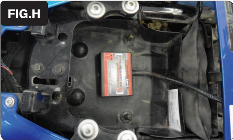
14 Using the supplied velcro, secure the PCV inside the tail section as shown in Figure H.
