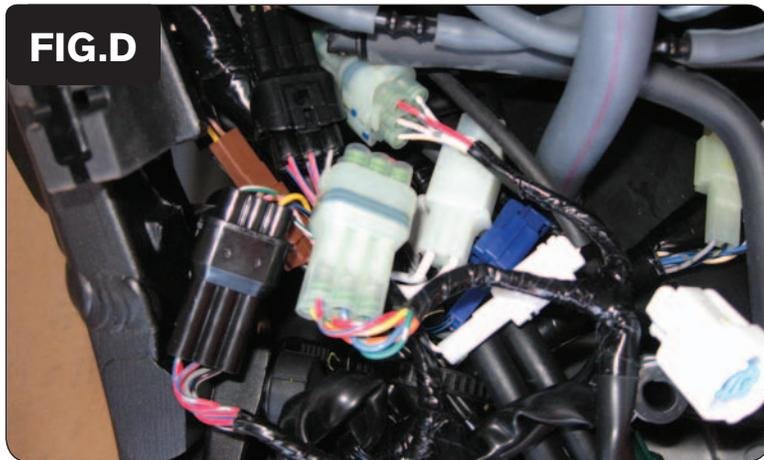
8 Plug the PCV connectors in-line of the throttle bodies and main wiring harness (Fig. D). Plug the colored connectors from the PCV into the matching stock connectors.
