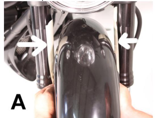
squeezing the fender above the fatter bottom portion of the fork tubes.
