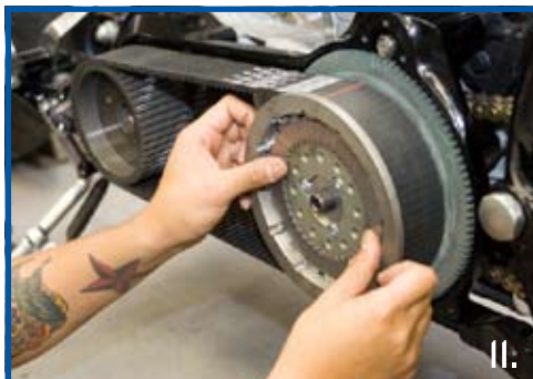
Apply the clutch basket, front pulley and belt. Carefully grease the supplied ball bearing and install into transmission shaft.
