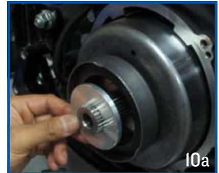
Place the front pulley spacer onto crankshaft and spring spacer onto front pulley.
