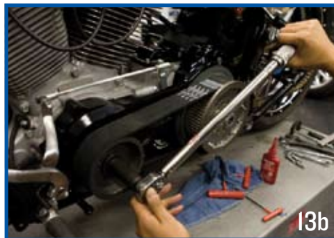
Tighten the supplied compensating sprocket bolt with both the supplied and the stock washers (13a) to 155 to 165 ft-lbs with thread locking compound (13b).
