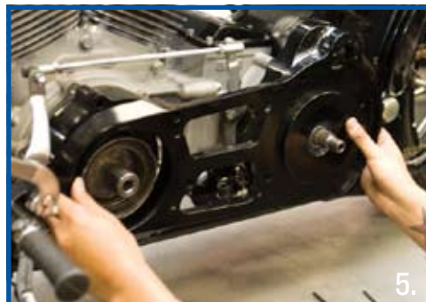
Following the components drawing included in the instructions, attach the backing plate with the specified hardware listed on the drawing. NOTE: The use of thread locking compound is highly recommended on the specified hardware when attaching the backing plate
