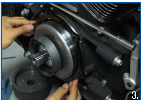
Remove the OEM Gasket and place supplied motor spacer.
