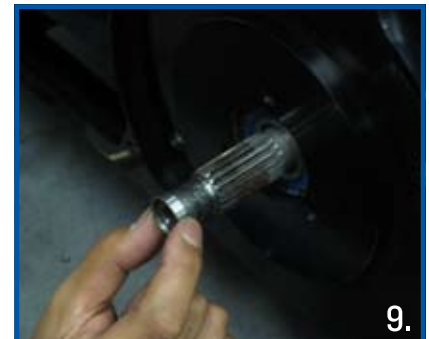
Place clutch spacer onto the transmission input shaft
