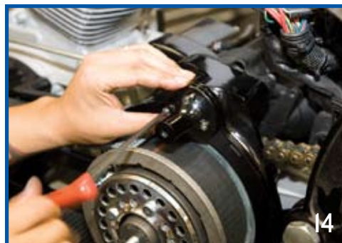
Apply the spring plate cover with the shoulder bolts and the starter cone using the 3 supplied 1/4-20 bolts (use thread locker and torque spring plate bolts to 25 to 30 ft-lbs and the starter cone bolts to 6-10 ft-lbs
