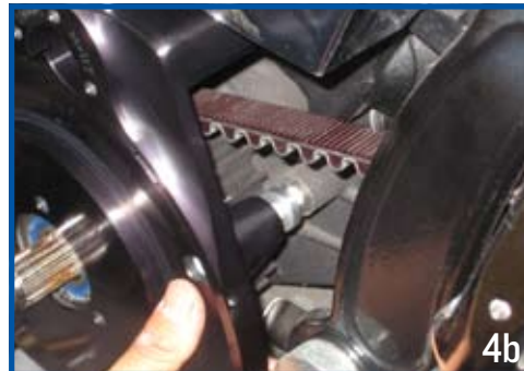
Place inner primary against motor spacer (4a) and capture transmission housing spacers between transmission and inner primary (4b).
