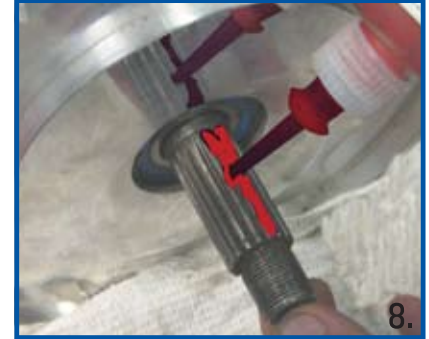
Before applying the clutch basket and components, the use of thread locking compound is required on the transmission main shaft. NOTE: Not using thread locking compound will void any warranty with PM/BDL
