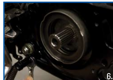
Before applying the clutch basket and components, the use of thread locking compound is required on the transmission main shaft. NOTE: Not using thread locking compound will void any warranty with PM/BDL
