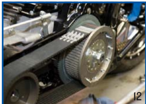
Apply the main shaft nut and torque to 70 to 80 ft-lbs
