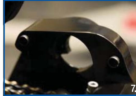
7. Install the electric starter using the supplied bolts NOTE: Use of the 2 alignment dowel pins located between the starter and primary are required
