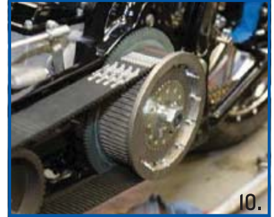
10. Apply the main shaft nut and torque to 70 to 80 ft-lbs
