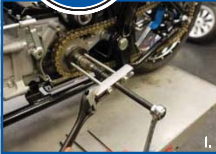
1. Using an Inner Bearing Race Remover, completely remove the inner bearing race located on the transmission main shaft
