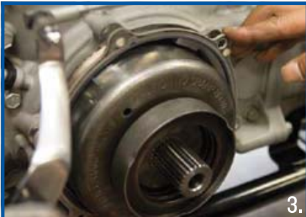
3. Use of the OEM gasket between the motor and primary is required for the PM primary. Install the PM Backing plate
