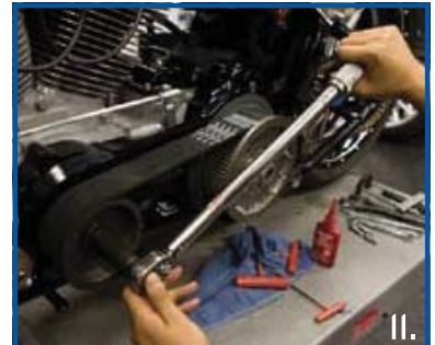
6. Tighten the compensating sprocket bolt to 155 to 165 ft-lbs with thread locking compound
