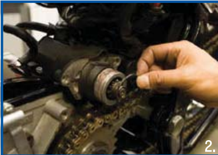
2. Remove the rubber O-ring located on the electric starter to ease the installation of the backing plate in the following steps
