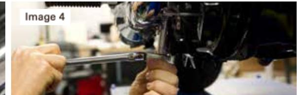
6. Remove bolt that attaches muffler to mounting bracket. **(Reference image 5)**
