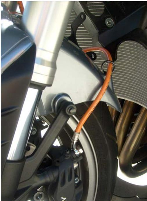
**g. LINE C - Left caliper, notice OEM routing tabs**
