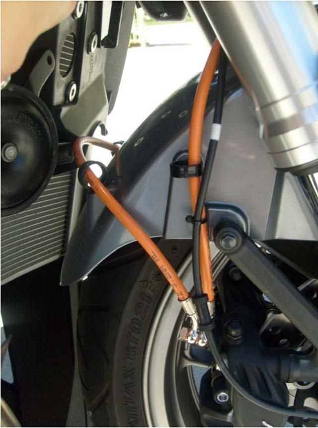
**e. LINES B & C – Right caliper, notice OEM routing tabs**
