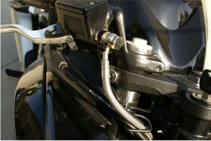
**a. Front master cylinder, notice the routing**
