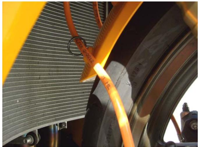
**d. Galfer line routed through OEM holder at fender**
