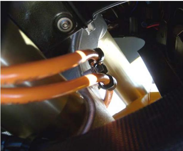
**c. Galfer c-clips at lower triple tree**
