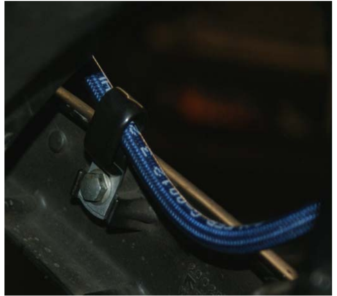
B. Galfer C-Clip on Swing Arm
