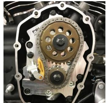
14. Install lifters, pushrods and rocker arms, Feuling recommends using an oil squirt can to manually pump up the lifters, pushrods and rocker arms during assembly. This will aid in lubrication for initial start up and will provide a quiet engine with immediate oil psi.
