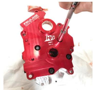
8. Rotate oil pump gears so gear flats are vertical to match the crankshaft per step 6. We found having the crank and gear flats vertical make for the easiest install of the oil pump and camplate assembly.
