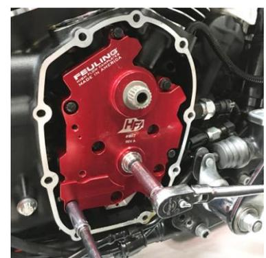
10. With the oil pump and camplate bolts finger tight rotate the engine over by hand, tighten and torque the camplate bolts first then the oil pump bolts, this process will center the camplate and pump as best as possible to the engine and crankshaft runout. Alternately step torque camplate and oil pump bolts up to a final 120 inch pounds.
