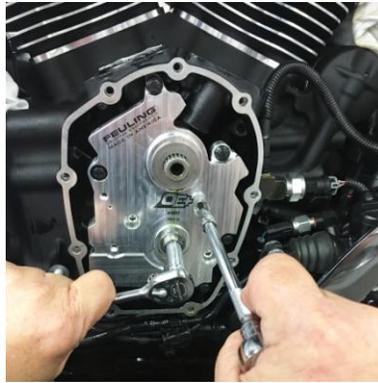
12. Install sprockets, lining up timing marks. Check sprocket alignment with a straight edge, use correct thrust washer thickness to achieve proper sprocket alignment. See Feuling #8041 for spacer thickness selection/options. Sprocket alignment is critical for wear and longevity of tensioner pad.
