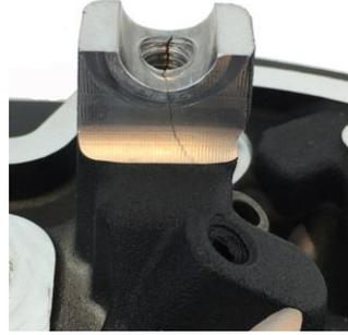
\*FEULING Rocker Stud/Nut kit #3047 will reduce stress on the rocker arm head stand offs. The rocker arm 'stand offs' are a weak link and prone to cracking.
