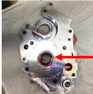
Rotate pump gears so flats are vertical to match crankshaft
