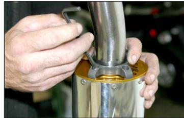
5. Install the O2 sensor (if applicable) into the new slip tube. If your bike does not require an O2 sensor, use the supplied aluminum block off bolt and copper washer to seal the threaded O2 bung in the slip-on tube. Do not over tightened the O2 sensor, refer to the Honda shop manual for proper torque specification. Slide the slip-on connector pipe onto the end of the headers, using the stainless steel Barrel clamp to attach it to the headers. Leave loose for now.
