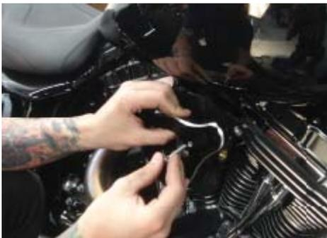
5. Torque breather bolts(6) to 15 ft-lbs. 6. Install rubber oil tubes. **Note: Oil tubes are not used on Sportster models**
