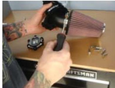
3. With the filter removed clean according to K&N's filter cleaning instructions which are included in the filter care service kit. K&N's filter care service kit can be purchased from K&N directly or almost any automotive parts store. Go to [www.kandn.com/cleaning.htm](http://www.kandn.com/cleaning.htm) for cleaning instructions.
