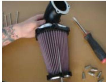
2. Slide the aluminum rear filter cover (14) off the filter onto the 90degree tube (12) to expose the hose clamp (15). **Tip: Place masking tape around the 90degree tube (12) to protect the finish from damage!** Loosen the hose clamp to free the filter element (16).
