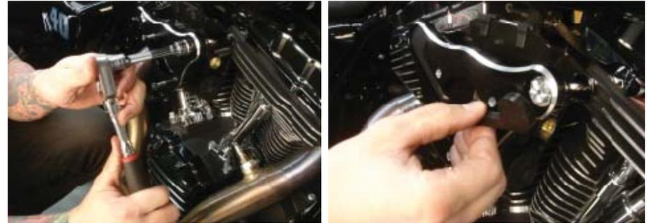
7. On Big Twin & Sportster models using the supplied 1/4"-20 x 3/4" socket head bolts(10) install the secondary plate(8), gasket(11), and complete filter assembly(9) and torque to 8 ft-lbs. On 2008-up FL models with electronic throttle install the secondary plate(8), gasket(11), and complete filter assembly(9) using the 1/4"-20 x 1-1/4" socket head screws and torque to 8 ft-lbs.
