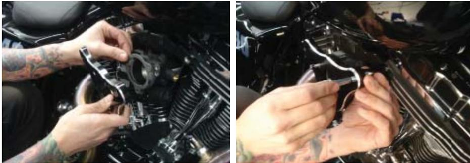
4. On Big Twin & Sportster models attach the backing plate(4) to the carburetor/throttle body using the supplied 1/4"-20 x 5/8" socket head bolts(5) and tighten to 8 ft-lbs. On 2008-up FL touring models with electronic throttle locate the backing plate(4) to the throttle body using the supplied 1/4"-20 x 1-1/4" socket head screws. Do not tighten during this step.
