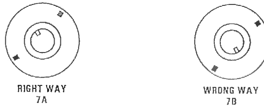
LOCATING PIN POSITION AT T.D.C. FOR SPORTSTERS
