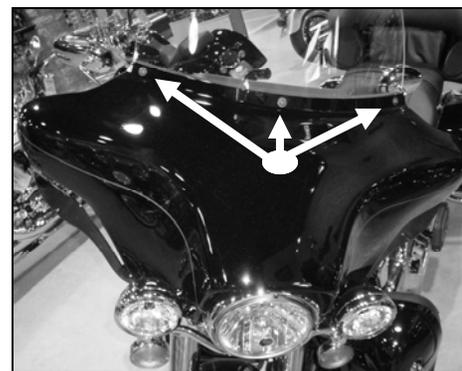
**Step#2:** Slide the lower, backing portion of the windshield bag down between the inner dash and the windshield. *Note: If using the USB cable option, you may need to loosen all 7 fairing screws to allow the outer fairing to pull back far enough to get the “U” around the top lip of the inner fairing as shown in Fig 1.3. Once the bag is in place, take any slack out of the loop.*
