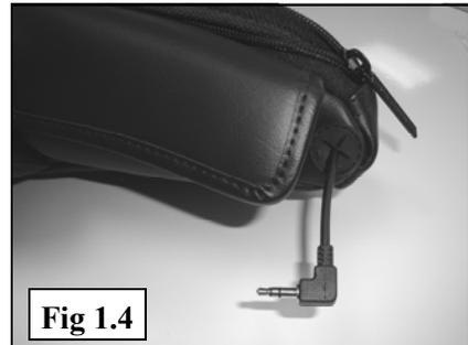
Make a “U” as shown in Fig 1.3. This allows your USB to go around the top lip of your fairing when installing the bag. On the far right of the bag is a 2nd “X” grommet that allows Hogtunes audio cable to pass out of the bag to the “aux in” on the radio. With USB power, and the audio out to the aux in, the zipper pouch is the ideal place to have your audio device for long rides!
