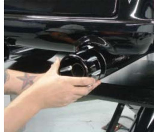
7. Reinstall the four 1/4"-20 bolts using red loctite and torque to 7 ft-lbs.
