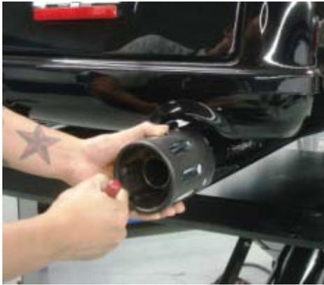
4. Once the four bolts are removed remove the exhaust tip.
