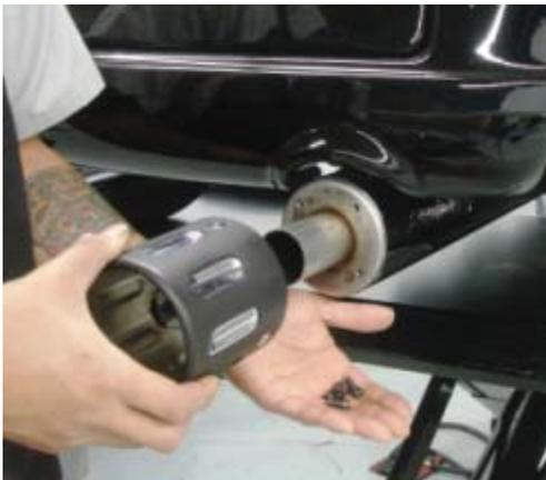
5. With the original exhaust tip removed reinstall the Performance Machine Elite exhaust tip. Align the Performance Machine Logo vertically and make sure the 4 bolt holes line up.
