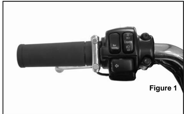
Route the wires from the dual button handlebar control bracket neatly along handlebar into the top fork tree area or inside the handlebar into the top fork tree area. From there run the wire assembly under the frame towards the battery. Alongside the battery or behind the left side cover is the approximate location that the control module will be mounted. Make sure to secure the wires along their routing with wire ties provided. Excess wire can be coiled and hidden in the battery area.
