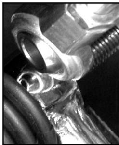
The rod end on the cylinder should be able to go past the point of mounting in each direction sideways. (Or shaft binding will occur). The point of mounting is the flat surface upon which the rod end
