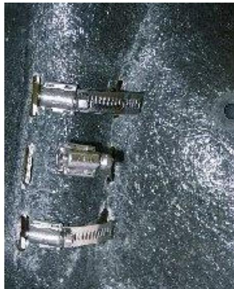
The clamps are inserted from the inside of the fairing using the slots closest to the headlamp tunnel, around the fork tubes and back into the inner so the worm drives are hidden inside the fairing when it is all assembled. The clamps get tightened to 20-25 inch pounds (1½-2 ft lbs). Over-tightening will only damage the fiberglass and won't add any strength to the installation.
